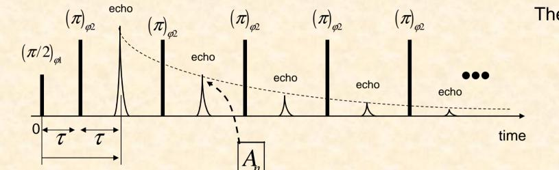
The echo train attenuation in heterogeneous samples
